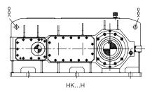
⚠ Note: Forbid to use the shaft end screw as the hoisting point after it is installed with hoisting ring.
