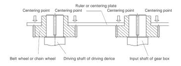
When installing belt wheel or chain wheel, ensure belt wheel and chain with certain tonus.
